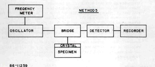
Figure 23 BLOCK DIAGRAM FOR RESONANCE TECHNIQUES
